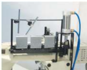
Foot lift by air or electricity, no noise, more sensitive response, sewn more efficient and the work is more comfortable
